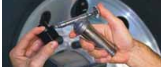
STEP 6 Lubricate each nut with one drop of oil between the nut and washer. Rotate the washer to distribute the oil evenly.
