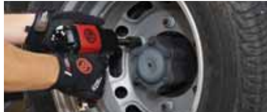
STEP 8 Use a CP7748 impact wrench on the lowest torque setting to quickly snug all the nuts prior to final torquing.
