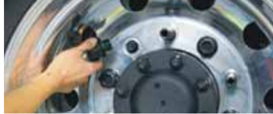
STEP 7 Install the nuts by hand.
