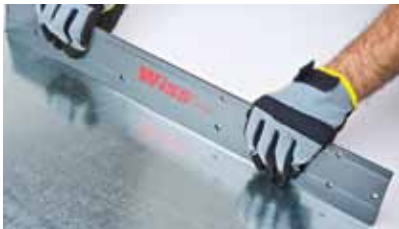
Ideal for making long, uniform bends. Also permits 180° bends for folding drive cleat channels.
